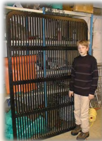
The most popular deep sea grid, a Norwegian produced 19 mm steel grid (1.3x2.5 m).
