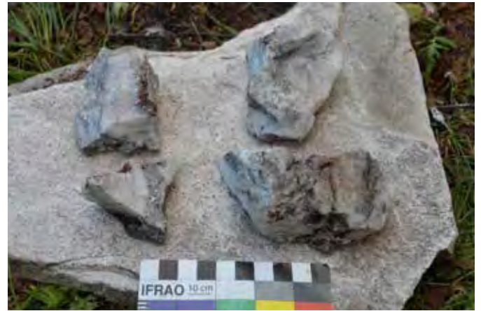
Figur 148 Greyish chert pieces (B2, before, left, and after burning). They burnt in the middle of the fire for about half an hour, at a presumed c.500°C. All the pieces got milky white. Two pieces were shock-cooled by water. They did not implode. Reddish material on pieces prior to firing may stem from prehistoric fire-setting
