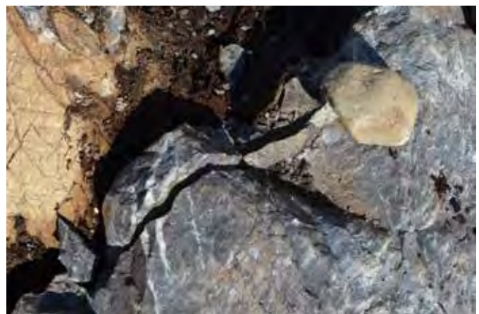
Figur 168 After much percussion bits and pieces eventually broke loose. Test site B
