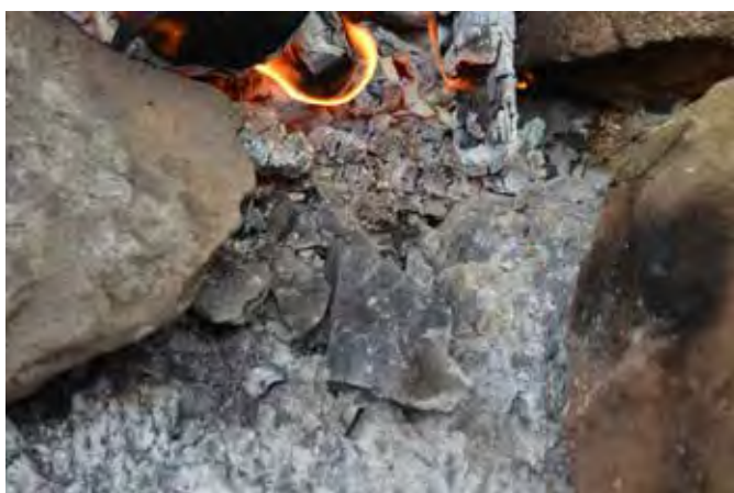
Figure 153 Early cracking of chert into small pieces unusable for tool production, after some 10-15 minutes, LAB1. Note that the chert has not become milky white, implying that the temperature will have been c. 3-400°C
