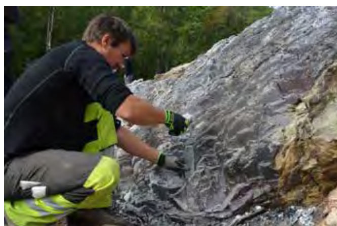
Figur 162 Using a stone wedge to loosen a piece of chert along a tight crack induced by fire-setting (LAB3)
