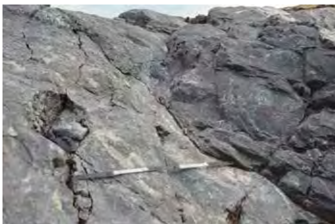
Figur 126 Close up of part of Zone 2, with convex surfaces at the right (es13 in the survey map). These are probably a result of fire-setting.
