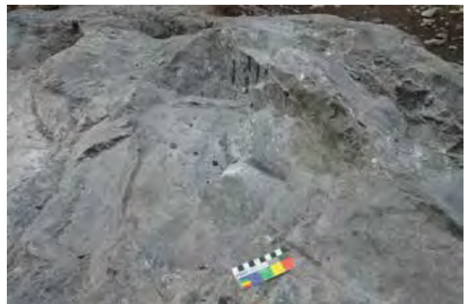
Figur 164 The final forms in the bedrock at LAB2 after fire-setting and cleaning. Note how the convex forms "stop" by the ledge
