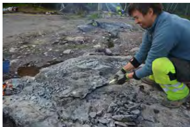
Figure 154 Deeper crack formed between two fires with a resulting slab weighing 20-30 kilos (LAB2)
