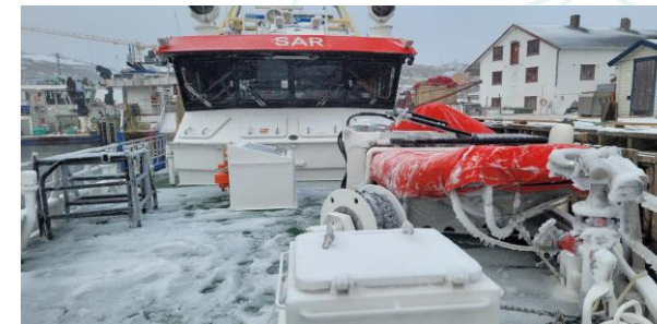
26 April 2022. Spray and snow icing. Photo: Redningsselskapet
